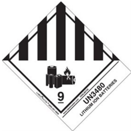
Class 9 Label (UN3480) Lithium Ion Batteries "Standalone"
